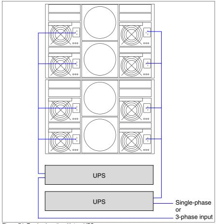
Figure 74: Two basic units with two UPSs
